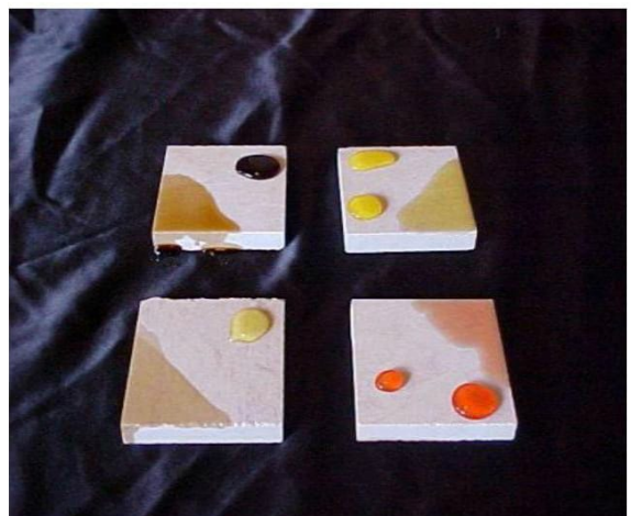
Above Left: Photo demonstrating water beading on sealed grout line Above Right: Photo showing partly sealed/unsealed Limestone
